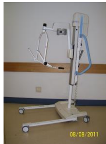
ArjoHuntleigh Older MaxiMove Hoist SWL: 190 kg Location: Rehab and PCU
