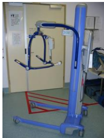
ArjoHuntleigh MaxiMove Hoist SWL: 228 kg Location: QuEST, AICU, 2D, Gem, ECU and CAM
